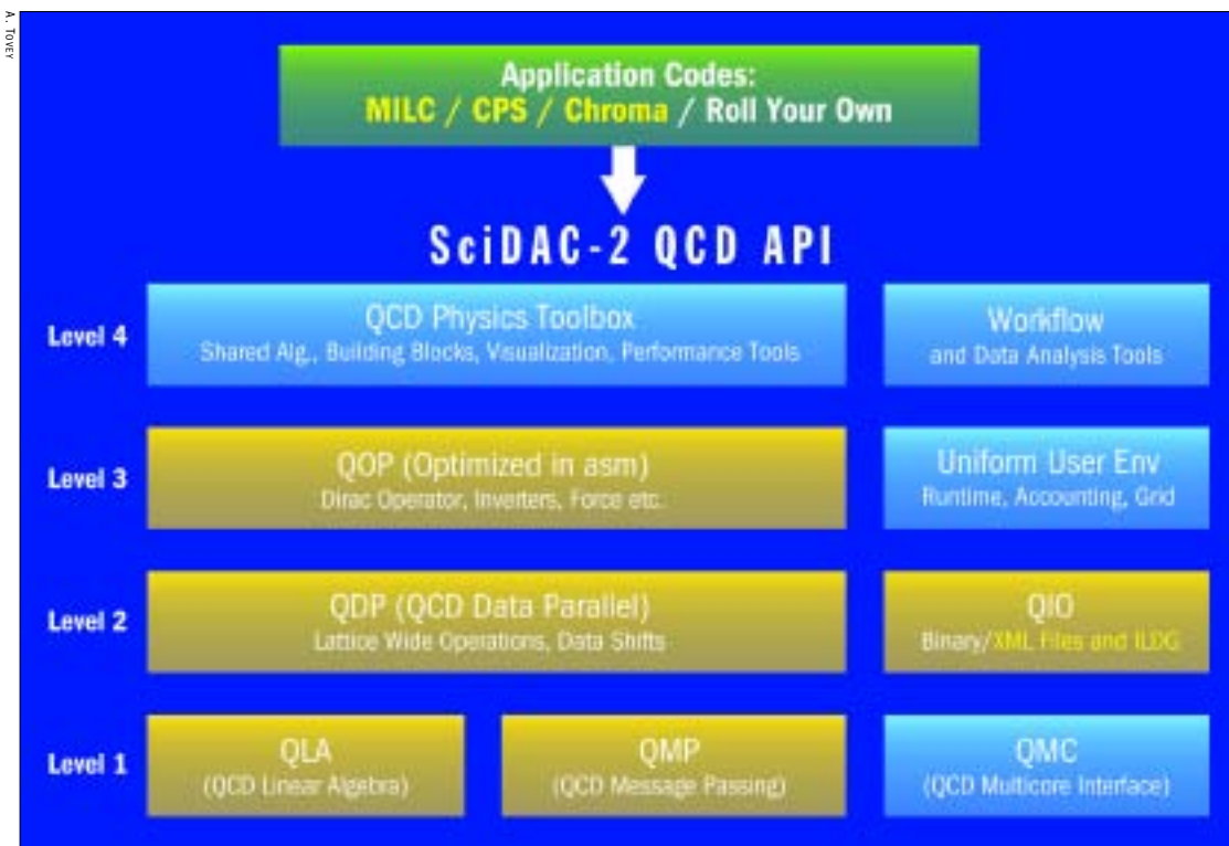
Figure 10. The SciDAC QCD API. SciDAC-1 components are shown in white lettering, and the new SciDAC-2 components in yellow lettering.
